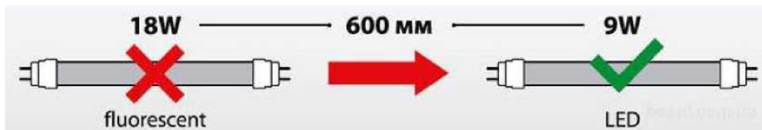
Figure 1 - Replacement of tubular fluorescent lamps with LED analogues
