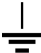
Figure 1 - Earth electrode identification mark
